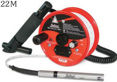
The 122 Mini is a convenient small version of the Solinst Interface Meter, small enough to fit in a backpack. A custom carrying bag is also an option. The Mini is available in 65 ft. or 20 m lengths.
