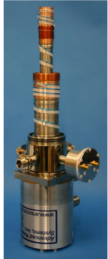
The above picture shows a cryocooler with no vacuum shroud or radiation shield. A bulkhead with 2 SMA connectors are shown. This has the upgrade instrumentation skirt.
