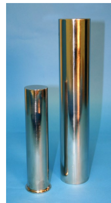
The above picture shows the vacuum shroud and radiation shield for the cryostat.
